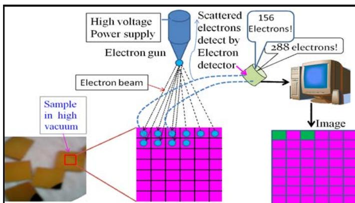
**Figure 5:** is the schematic diagram SEM imaging technique that how electrons is emitted from the surface of our Hydrogenated Diamond Like Carbon to the detector for the formation of SEM image.
