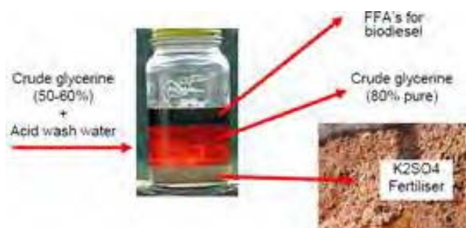
Figure-3: The Traditional Method of Removing Glycerol(Fraunhofer, n.d.-a)
