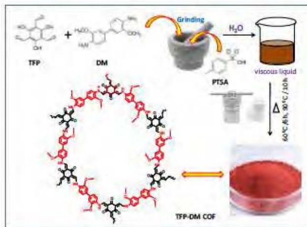
Figure 13: Production Procedure of TFP-DM COF Nano-sheet Catalyst (Chowdhury et al., 2020)
